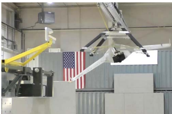
Figure 5 | DARPA's SideArm research effort seeks to create a self-contained, portable apparatus able to horizontally launch and retrieve unmanned aerial systems (UASs) of up to 900 pounds. Photo courtesy of DARPA.
