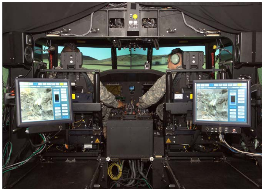
Figure 2 | Flight2 transformed a federated system – one using distributed avionics functions packaged as self-contained units – into a modern digital system by providing commonality with commercial aircraft. Credit: Rockwell Collins.
